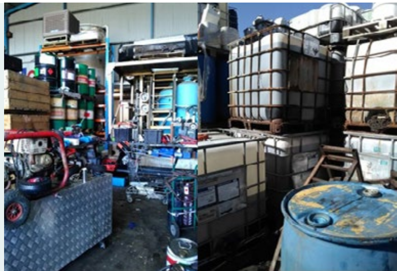
A number of hazards can be identified from the two images, including inadequate packaging of corrosives and flammable liquids co-located with ignition sources
